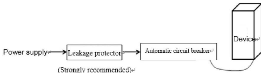
Connect the device to the automatic circuit breaker first and then to the power supply, see the diagram above.
